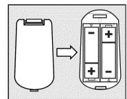
2 Open the battery compartment, insert the batteries as shown and then close the battery compartment. Match the polarities (+ and -) on the batteries with the diagram on the remote.
